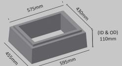
Concrete surround for around yellow fire hydrant cover. Typically set into the road or footpath
